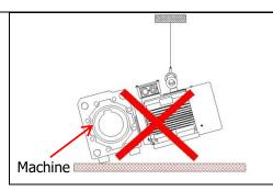
**Caution:** the lifting eyebolts are sized for lifting only the motor, brake and auxiliary components, if any, therefore **they must not** be used for lifting the motor when it is connected to other machines.
